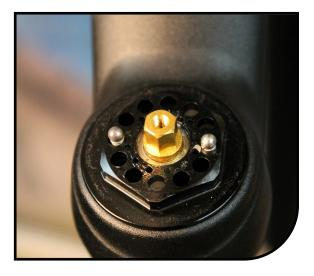
2 Unthread ABS+ compression damper assembly from the stanchion using a 24mm socket and ratchet. If the fork has the Kwik Toggle compression damper you will need to use the Manitou Cassette Tool and 1" wrench or socket to remove the damper.
