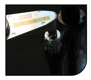
10 Install air spring assembly into stanchion. Using a 22mm crow's foot, tighten assembly end cap to 80-100 in lb [9.0-11.3 N m].
