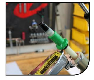
11 Attach a shock pump and inflate air leg to 40-50PSI. This will aid in installing the casting later.
