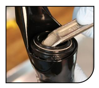
5 Using a downhill tire lever or similar tool, gently pry the dust seals out of the casting.
