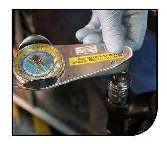
5 If installing an ABS+ damper use a 24mm socket and torque wrench, tighten the damper to 60–80 in lb [6.8–9.0 N m].
