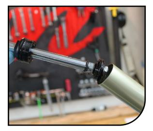
Install rebound damper into stanchion. Using a 22mm crow's foot and torque wrench, tighten the rebound damper assembly end cap to 80-100 in lb [9.0-11.3 N m].
