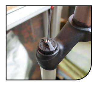
8 Clean fork and use a shock pump to set to desired pressure. Pressure charts on next page for reference.
