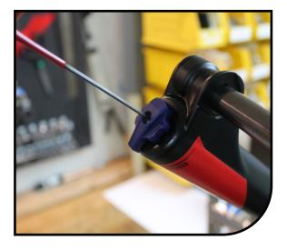
8 Install compression rod bolt. It helps to have at least 50psi in the air chamber when tightening down the bolt to the proper torque. Use a 12mm socket and torque wrench and tighten to 45–55 in lb [5.1–6.2 N m].
